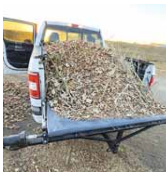
Remote-control Bed Boss connects directly to the truck battery or an accessory wire.
