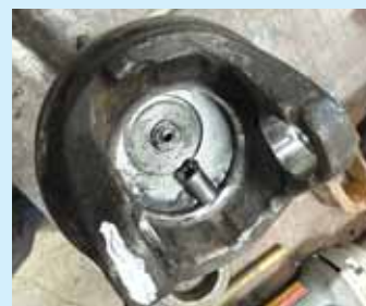
Photo shows peg broken off, about 1 in. long, 1/2 in. in diameter, with a 3/16-in. hole in the center for grease.
