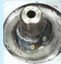
Photo shows peg broken off, about 1 in. long, 1/2 in. in diameter, with a 3/16-in. hole in the center for grease.
