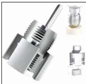
Tool features a clockwise cutting action that cleans or rethreads damaged or blocked pipe threads. It can cut and repair both internal and external threads on 1/2-in. and 3/4-in. pipes.
