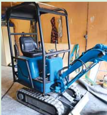
Mini excavator with weather enclosure frame before add-ons.
