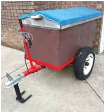
An electric actuator makes lifting and dumping the 22 by 42 by 20-in. high wagon easy.
