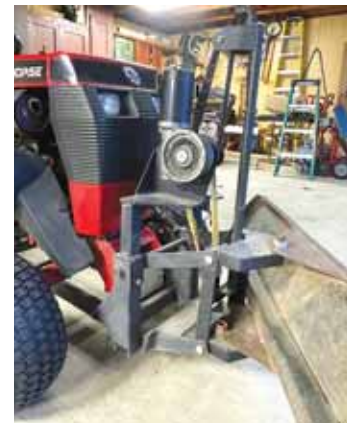
Carra modified a front blade from an older Craftsman garden tractor for use on the Wheel Horse.
