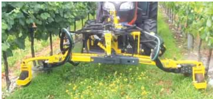
“Tap water is sprayed through rotating nozzles at 14,500 psi, destroying the weeds by stripping the collar and disrupting the root system,” says Staker.
